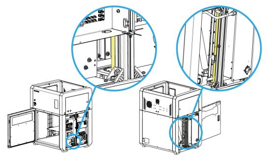
Once you have applied the grease to both leadscrews, turn on the printer and move the build plate up and down all along the printing area.
