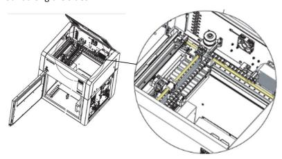
Move the printhead all over to lubricate the guidelines properly.
