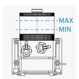
**5.** Once the reservoir is loaded, turn on the machine. The system will begin to purge the remaining air in the system and the user will see that the level drops. You will need to add more liquid to reach the max level. Repeat this operation until you see the max level is stabilizing. After this procedure, close the reservoir and open the small cap, and leave it open.
