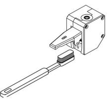
**3.** Using a brush, gently clean the inside of the Bowden and the gears. Removing any residue will improve the grip of the extruder and will minimize the risk of cross-material contamination when printing.
